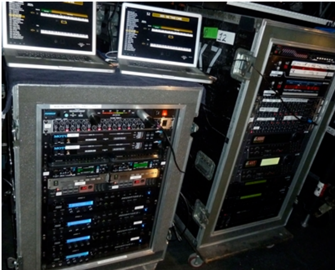
Roy Bittan's understage rig: The rack on the left is the new system with duplicates of everything as spares. The rack on the right is the old system which is no longer in use
